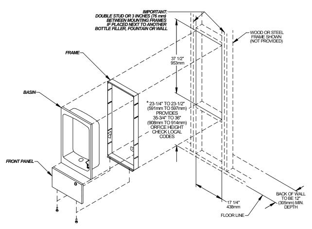
\* These dimensions are required to obtain proper rim and bubbler heights for compliance with ANSI standard A117.1.
